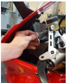
1. Under the mirror inside the fairing remove 2 bolts that hold the mirror in place
