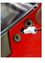
3. Feed the mirror block wire into the center hole. It may be a tight fit depending on your bikes piticular manufacturing tolerance. Feed it through with the little clipy part facing the center line of the bike. it may help to pull from the underside
