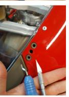
\*\*\* On some bikes the fairing hole trimming isn't as consistent from the factory. You may need to skim the edge with a deurring tool or sharp knife to clear the mirror blocks. Carefully trim a little at a time and check often until it fits
