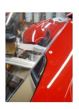
When installing the fasteners leave everything loose until both bolts are threaded you may need to wiggle things around to get alignment all depending on you particular bikes manufacturing tolerance and fit.
